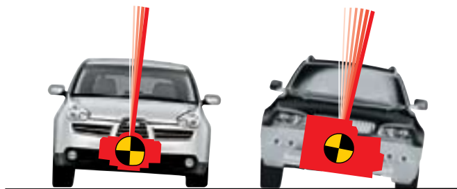
The SUBARU BOXER engine's lower centre of gravity causes less body roll than an in-line or V-type engine.
