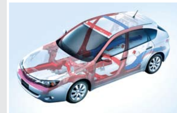
Advanced ring-shaped reinforcement frame
