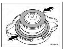
3. After refilling the reserve tank and the radiator, reinstall the caps and check that the rubber gaskets inside the radiator cap are in the proper position.
