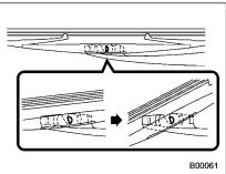
2. Turn the wiper blade assembly counterclockwise.
