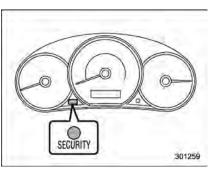
The security indicator light deters potential thieves by indicating that the vehicle is equipped with an immobilizer system. It begins flashing (approximately once every 3 seconds) approximately 60 seconds after the ignition switch is turned from the "ON" position to the "Acc" or "LOCK" position or immediately after the key is pulled out.
