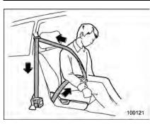
The driver's and front passenger's seatbelts have a seatbelt pretensioner. The seatbelt pretensioners for the driver's seat and front passenger's seat operate at the same time as the frontal, and side SRS airbags. If the vehicle rolls over, they operate simultaneously with the curtain airbag.
