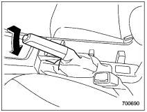
To release the parking brake, pull the lever up slightly, press the release button, then lower the lever while keeping the button pressed.
