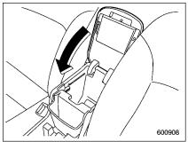
1. Tip the console top forward from its vertical position.
