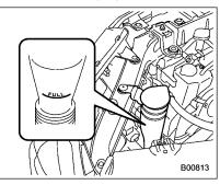
Remove the washer tank filler cap, then check the fluid level indicated by the level gauge (attached to the inside of the cap). If the level is near the "Low" mark, add fluid until it reaches the "Hi" level on the level gauge or the "FULL" mark on the tank.
