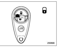
Press the "" button to lock all doors and the rear gate. An electronic chirp will sound once and the turn signal lights will flash once.
