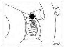
Push the "RES/ACC" button and hold it until the vehicle reaches the desired speed. Then, release the button. The vehicle speed at that moment will be memorized and treated as the new set speed. When the difference between the actual vehicle speed and the set speed is less than 4 mph (6.8 km/h), the set speed can be increased 1 mph (1.6 km/h) each time by pressing the "RES/ACC" button quickly.
