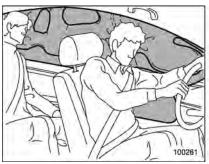
The SRS side airbag and SRS curtain airbag can function only when the ignition switch is in the "ON" position.
