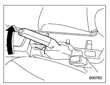
Check the parking brake stroke according to the maintenance schedule in the "Warranty and Maintenance Booklet". When the parking brake is properly adjusted, braking power is fully applied by pulling the lever up 7 to 8 notches gently but firmly (approximately 45 lbf [200 N, 20.4 kgf]). If the parking brake lever stroke is not within the specified range, have the brake system checked and adjusted at your SUBARU dealer.
