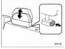
To raise the head restraint, pull it up. To lower it, push the head restraint down while pressing the release button on the top of the seatback. The head restraint should be adjusted so that the center of the head restraint is closest to the top of the occupant's ears. When the seats are not occupied, lower the head restraints to improve rearward visibility.
