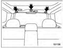
The tether anchorages (upper anchorages) are provided at the locations shown in the above illustration.
