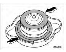
7. Put the radiator cap back on and tighten firmly. At this time, make sure that the rubber gasket in the radiator cap is correctly in place.
