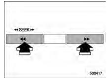
If you press the " $\blacktriangleleft$ " or " $\blacktriangleright$ " side of the SEEK button briefly, the radio will automatically search for a receivable station and stop at the first one it finds. This function may not be available, however, when radio signals are weak. In such a situation, perform manual tuning to select the desired station.
