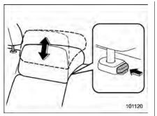
To raise the head restraint, pull it up while pressing the release button on the top of the seatback.
