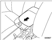
2. Push the armrest part of the console top forward to the desired position. Adjust the position of the armrest to suit your
