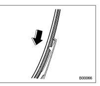
4. Align the claws of the plastic support with the grooves in the blade rubber assembly, then slide the blade rubber assembly into place.
