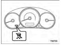
This single light has the function of indicating malfunctions in the Vehicle Dynamics Control system and the function of indicating that the Vehicle Dynamics Control system is not operating. It illuminates in the event of a malfunction in the system and is illuminated whenever the system is not operating.  $\bigtriangledown$  Vehicle Dynamics Control warning light
