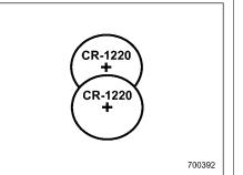
2. Remove the circuit board from the bottom half of the case and slide the white plastic battery holder out from under the battery tab releasing the batteries. Remove the old batteries and replace with new ones. Be sure to observe the (+) sign on the old batteries before removing them to ensure that the new batteries are inserted properly (battery "+" should be pointed away from the transmitter circuit board on both batteries).
