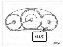
A diagnostic system continually monitors the readiness of the SRS airbag system (including front seatbelt pretensioners) while the vehicle is being driven. The SRS airbag system warning light "AIR-BAG" will show normal system operation by lighting for approximately 6 seconds when the ignition switch is turned to the "ON" position.
