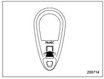
A "PANIC" button is located on the back of the transmitter.
