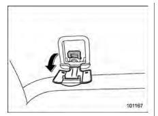
2. For both window-side seating positions, remove the cover for the appropriate upper anchorage.
