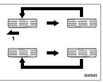
Vehicles equipped with unidirectional tires 1) Front
