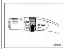
The front fog lights operate only when the low beam headlights are illuminated.
