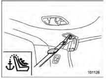
Attach the child restraint top tether hook to the appropriate upper anchorage.
