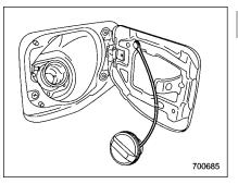
3. Hook the cord that is attached to the fuel filler cap onto the hook inside the fuel filler lid.
