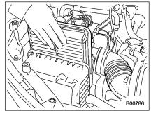
4. Open the air cleaner case cover and remove the air cleaner element.
