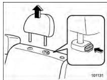
1. Remove the headrest at the windowside seating position where the child restraint system has been installed with the lower anchorages or seatbelt; lift up the headrest while pressing the release button. Store the headrest in the cargo area. Avoid placing the headrest in the passenger compartment to prevent it from being thrown around in the passenger compartment in a sudden stop or a sharp turn.
