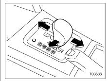
With the vehicle either moving or stationary, move the selector lever from the "D" position to the manual gate then move it to the "+" end or "-" end of the manual gate to select manual mode.
