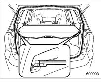
To extend the cover, pull the end of the cover out of the housing, then insert its hooks into the catches as shown. To rewind it, unhook it from the catches and it will rewind automatically. You should hold on to the cover and guide it back into the cover housing while it is rewinding.
