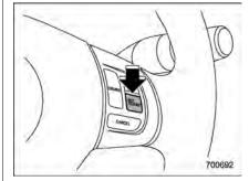
Push the "SET/COAST" button and hold it until the vehicle reaches the desired speed. Then, release the button. The vehicle speed at that moment will be memorized and treated as the new set speed.
