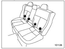
The lower anchorages (bars) are used for installing a child restraint system only on
