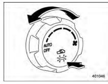
**ON position (Recirculation):** Interior air is recirculated inside the vehicle. Push the air inlet selection button to the ON position for fast cooling with the air conditioner or when driving on a dusty road. The indicator light will illuminate.
