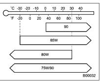
SAE viscosity No. and applicable temperature
