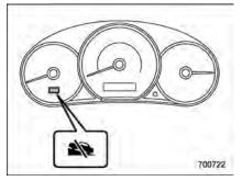
When the ignition switch is turned to the "ON" position, the Hill start assist warning light illuminates and turns off after approximately 2 seconds. While the engine is rotating, if any malfunction is detected in the Hill start assist system control, the warning light will illuminate. If the warning light illuminates, have the vehicle inspected by your SUBARU dealer.
