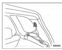
A coat hook is attached to each side of the cargo area.
