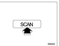
Press the "SCAN" button to change the radio to the SCAN mode. In this mode, under the selected category, the radio scans through the channel until a station is found. The radio will stop at the station for 5 seconds while displaying the channel number, after which scanning will continue until the entire channel has been scanned from the low end to the high end.
