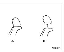
A) When not used (retracted position)B) When used (click position)
