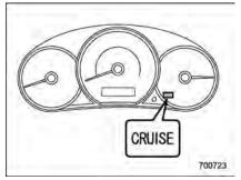
The "CRUISE" indicator light on the combination meter will illuminate.
