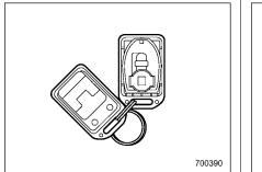
1. Carefully pry the remote control halves apart using a small flat-head screwdriver.
