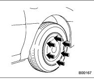
Align the valve with the valve hole in the cover, then fit the cover on the wheel by tapping your hand evenly around the circumference of the cover.
