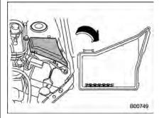
2. Pull any one spare fuse out of the spare fuse holder in the engine compartment. Spare fuses are attached on the back side of the fuse holder cover. You may pick up any one fuse in the spare fuse holder.
