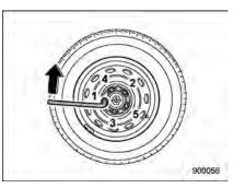
15. Use the wheel nut wrench to securely tighten the wheel nuts to the specified torque, following the tightening order in the illustration.
