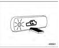
**ON position (Recirculation):** Interior air is recirculated inside the vehicle. Push the air inlet selection button to the ON position. The indicator light will illuminate.
