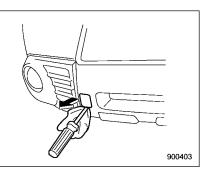
2. Pry off the cover on the front bumper using a screwdriver, and you will find a threaded hole for attaching the towing hook.
