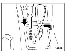
4. Insert the screwdriver into the hole.
