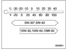
SAE viscosity No. and applicable temperature
