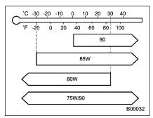
SAE viscosity No. and applicable temperature
