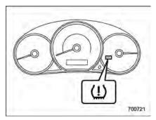
The tire pressure monitoring system provides the driver with a warning message by sending a signal from a sensor that is installed in each wheel when tire pressure is severely low.
