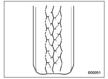
Rolling resistance is high, so fuel consumption is also higher. • Abnormally high tire pressure (tread worn in center)
