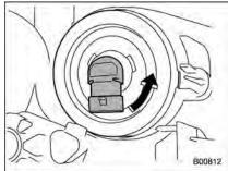
3. Remove the bulb from the headlight assembly by turning it counterclockwise.
