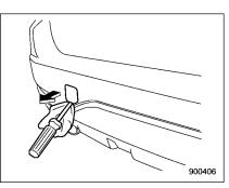
2. Pry off the cover on the rear bumper using a screwdriver, and you will find a threaded hole for attaching the towing hook.
