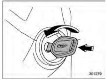
The key can be turned from "Acc" to "LOCK" only when the key is pushed in
