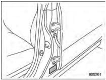
The certification label attached to the driver's side doorjamb shows GVWR (Gross Vehicle Weight Rating) and GAWR (Gross Axle Weight Rating).
