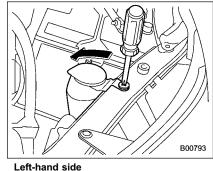
2. Use a screwdriver to remove the secured clip of the washer tank. To make it easy to access the bulb, move the washer tank to the horizontal direction (left-hand side).
