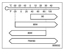
SAE viscosity No. and applicable temperature
