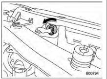
1. Turn the bulb socket counterclockwise and pull out the socket.
