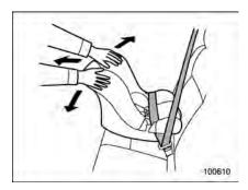
6. Push and pull the child restraint system forward and from side to side to check if it is firmly secured. Sometimes a child restraint can be more firmly secured by pushing it down into the seat cushion and then tightening the seatbelt.
