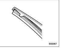
Securely retain both ends of the rubber with the stoppers on the plastic support
