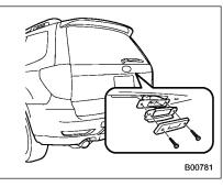
1. Remove the mounting screws using a Phillips screwdriver.
