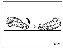
The SRS curtain airbags are not basically designed to deploy if the vehicle pitches end over end.
