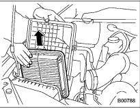
5. Open the air cleaner case cover and remove the air cleaner element.
