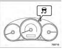
The indicator light illuminates when the ignition switch is turned to the ON position; it turns off approximately 2 seconds later. This indicator light flashes during activation of the skid suppression function and is illuminated steadily during activation of the traction control function.
