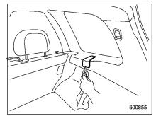
1. Remove the cover of the retainers by prying on the edge with a flat-head screwdriver.
