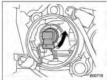
5. Remove the bulb from the headlight assembly by turning it counterclockwise.
