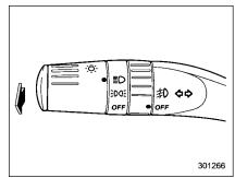
To change from low beam to high beam, push the turn signal lever forward. When the headlights are on high beam, the high beam indicator light " $\equiv$ O" on the combination meter is also on.
