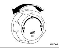
This dial is used to set the desired interior temperature. With the dial set to your desired temperature, the system automatically adjusts the temperature of air supplied from the outlets such that the desired temperature is achieved and maintained.
