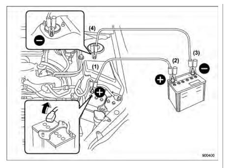
(1) Connect one jumper cable to the positive (+) terminal on the discharged battery.
