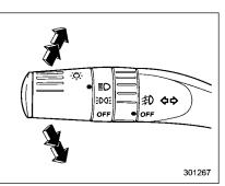
To activate the right turn signal, push the turn signal lever up. To activate the left turn signal, push the turn signal lever down. When the turn is finished, the lever will return automatically. If the lever does not return after cornering, return the lever to the neutral position by hand.
