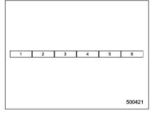
Presetting a station with a preset button allows you to select that station in a single operation. Up to six AM, FM1, FM2 and FM3 stations each may be preset.
