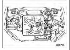
2. Pull out the level gauge that has the """ symbol on top, wipe it clean, and insert it again.
