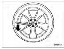
8. Loosen the wheel nuts using the wheel nut wrench but do not remove the nuts.
