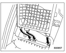
6. If the air cleaner case cover has been removed, insert the three projections on the air cleaner case cover into the slits on the air cleaner case.
