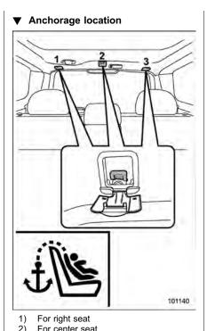
There are three anchorages for each seating position on the rear edge of the
