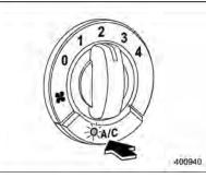
The air conditioner operates only when the engine is running.
