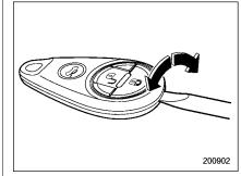
1. Open the transmitter case using a flat-
