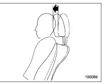
The front seats of your vehicle are equipped with active head restraints. They automatically tilt forward slightly in the event the vehicle is struck from the rear, decreasing the amount of rearward head movement and thus reducing the risk of whiplash. For maximum effectiveness, the head restraint should be adjusted so that the center of the head restraint is closest to the top of the occupant's ears.
