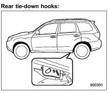
The rear tie-down hooks are located near each of the jack-up reinforcements.
