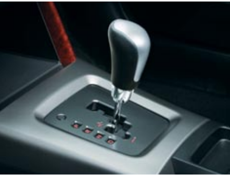
4-speed Electronic Direct Control Automatic Transmission with SPORTSHIFT™ (4EAT SS)
