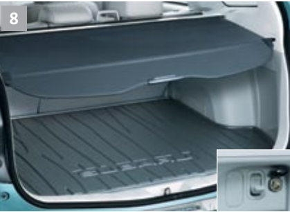
Cargo area: Tray, cargo hooks, 12-volt power outlet and retractable cargo cover
