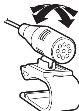
The microphone angle can be adjusted. □
