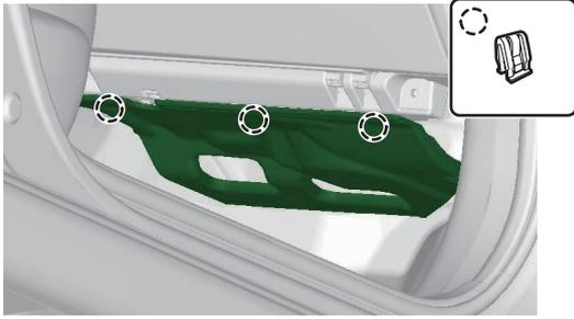
(18) Remove the under cover ASSY - passenger (manual A/C model) (Illustration 15).
