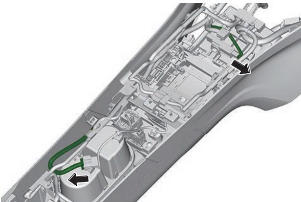
(8) Pull out the harness connector (models with hand brake) (Illustration 7).
