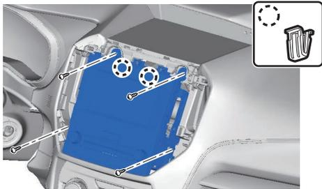
(16) Remove the audio or navigation system (for models with audio or navigation system) (Illustration 13).
