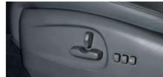
**Memory seat** - The eight-way power-adjustable driver's seat includes a memory feature that saves the precise seating preferences of two different drivers.
