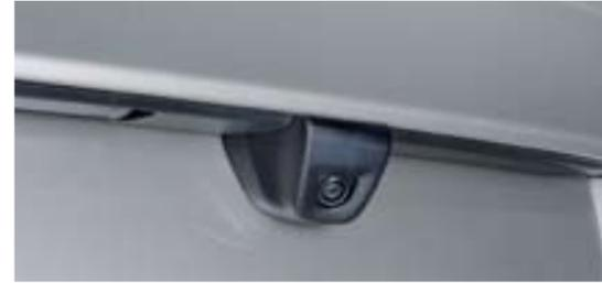
**Rear view camera** - This camera shows what's immediately behind the rear bumper on the monitor system. The monitor system also shows distance lines to help you back up safely.
