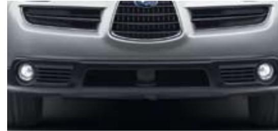
**Fog lights** - For those times when fog, snow or rain reduce visibility, multi-reflector halogen fog lights illuminate the road surface and bring added safety to the picture.
