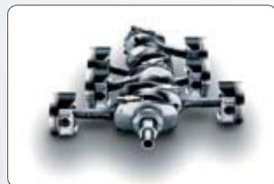
The horizontally-opposed engine, also known as the *boxer*, earned its nickname because its pistons move like a prize-fighter, alternately throwing left and right punches on a horizontal plane. The motion of the right bank of pistons counteracts that of the left bank, thereby balancing each other out and reducing engine vibration.
