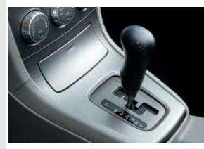
4-speed Electronic Direct Control Automatic Transmission
