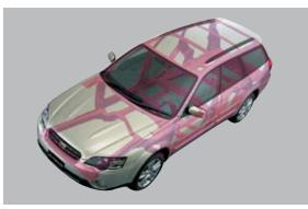
Advanced ring-shaped reinforcement frame
