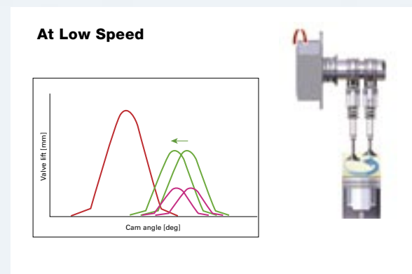
The fact that each intake valve is opened a different amount creates a swirl effect to better mix fuel and air, thus improving combustion, power and fuel economy.
