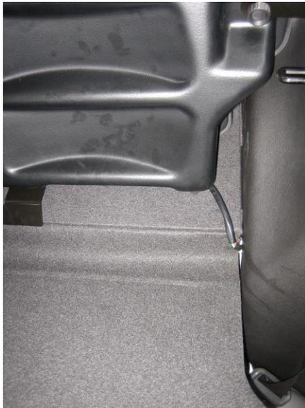
Put harness adapter and subwoofer connectors under carpet between rear seat and cargo floor.
