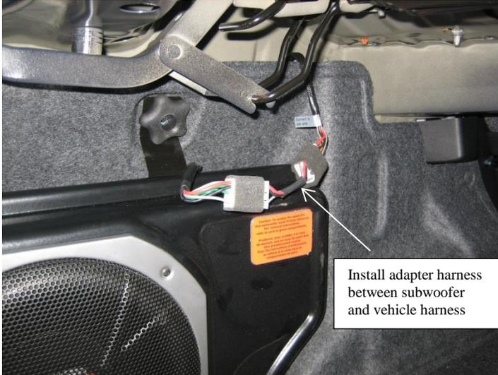
Install adapter harness in between subwoofer vehicle harness connector and subwoofer connector.
