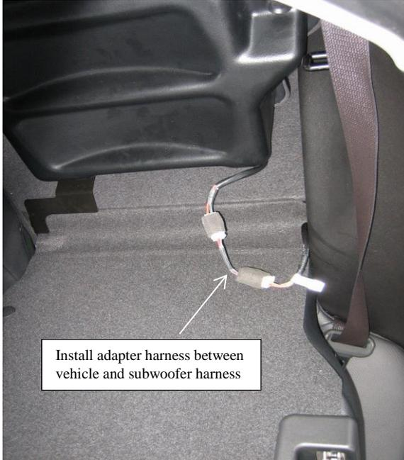
Install adapter harness in between subwoofer vehicle harness connector and subwoofer connector.
