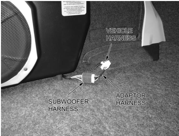
Install adapter harness in between subwoofer vehicle harness connector and subwoofer connector.
