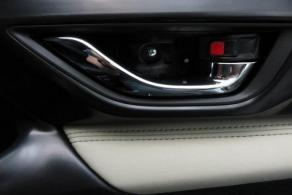
2: Remove the cover and screw that is located in the handle of the door
