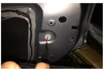
8: Unplug the connector located on the door panel
