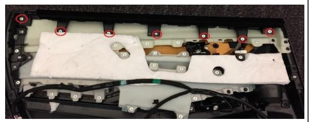
11: Undo the 7 clips holding the trim panel on by gently releasing the clip and pulling up on the trim.
