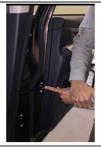
5: Grab the panel and pull out and lift up gently to release the door panel from the door
