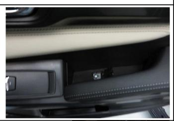
3: Use your fingers to pry on the top side of this plastic panel and pull it off (Note the clip locations)
