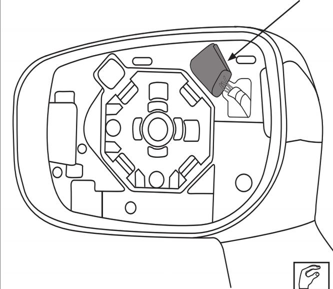
Locate and remove prearranged vehicle connector. (a)
