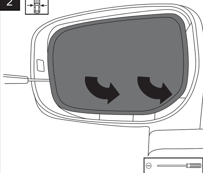
Protect mirror housing to prevent damage. Using screwdriver, remove mirror by disengaging the four mirror clips. Pull straight out to remove. Driver's side shown.
