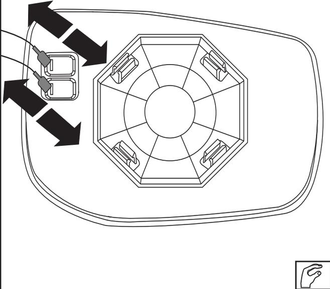
If equipped, disconnect heater terminals.
