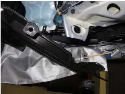
Remove 10mm self tapping screw and two expandable plugs from LH mud guard and swing mud guard out of the way.
