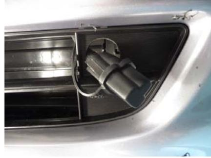
Using male plug protector, attach male plug to previously drilled hole in lower front grille.
