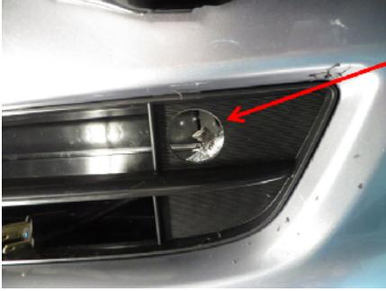
Using 32mm hole saw, drill hole in lower front grille in the location shown. Reference template on Page 5 for grille cutout.
