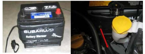
Wrap the warmer around the battery with the printed side facing outwards. Pull the warmer snug at the corners. Use the wire wraps provided to secure the warmer to the battery as shown. Install battery warmer around battery with wire exiting towards front as shown.
