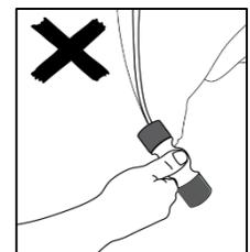
MAINTENIR EN PLACE LA PROTECTION DE BORD DE PORTE AVEC LA MAIN ET FRAPPER DIRECTEMENT ET FERMEMENT AU POINT DE FRAPPE N° 1.
